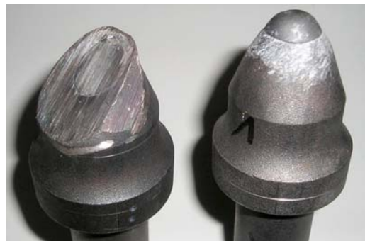
Fig. 2. An influence of a tangential rotary pick rotation decay on the edge wear, a laboratory tests result [5, 6]
