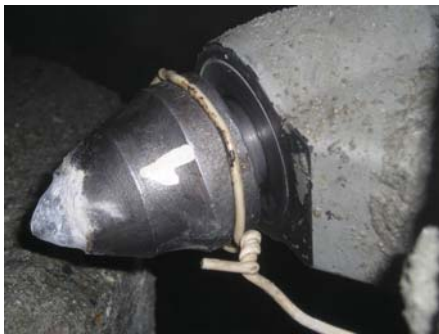
Fig. 11. A view of a tool edge and holder surface after tests of rock sample cutting at the length of about 1000 m, with holder water feed [6]
