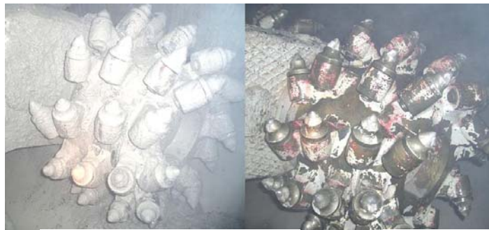
Fig. 15. View of the “dirty” cutting head of AM-50 roadheader with standard holders after mining (left) and the “clear” cutting head with lubricated holders after mining (right) [3, 6]
