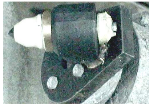
Fig. 6. Bearing of the tangential rotary tools with the supportive bearing globule in the holder [1, 2]
