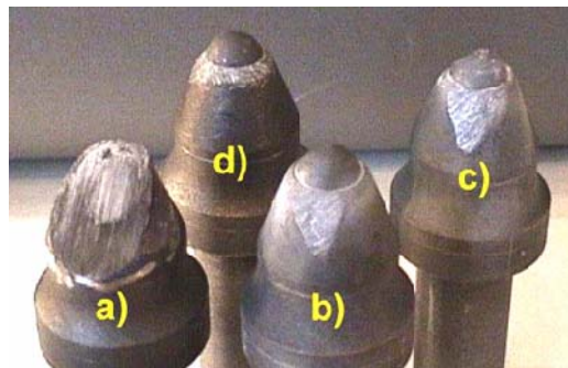
Fig. 12. The view of the rotary-tangential picks after the test along the length of ca. 2500 m: a) "dry" cutting; b) cutting with high pressure water jet assistance from front; c) cutting with rear high pressure water jet assistance; d) cutting in the lubricated holder, cutting depth 9 mm [3,6]
