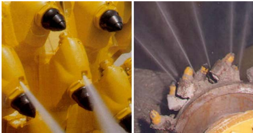
Fig. 4. A view of exemplary applications of high pressure assistance systems on roadheaders heads: on left – in the rear, on right- in the front [3, 6]
