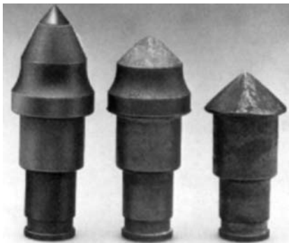
Fig. 1. An example of even wear of cutting tools obtained in laboratory conditions by the Krupp-Widia company [5, 6]
